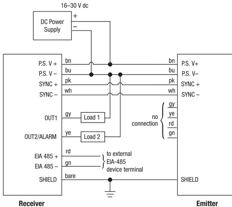
Receiver Output 1: (OUT1) is an open-collector transistor switch rated at 30 V DC maximum, 150 mA maximum. It is protected against overload and short circuits.
