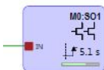
Figure 130. Safety output in Delay Off Timing mode
