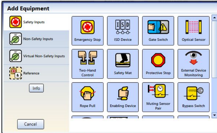
Figure 56. SC10-2: Adding inputs from Equipment View (physical status output can only be added from this view)
