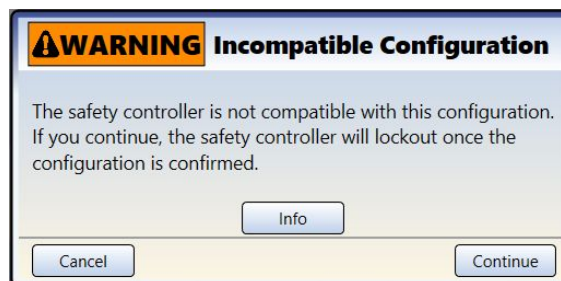
Figure 64. Incompatible Controller Warning
