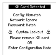
Figure 341. XS/SC26-2d Models: System Lockout
