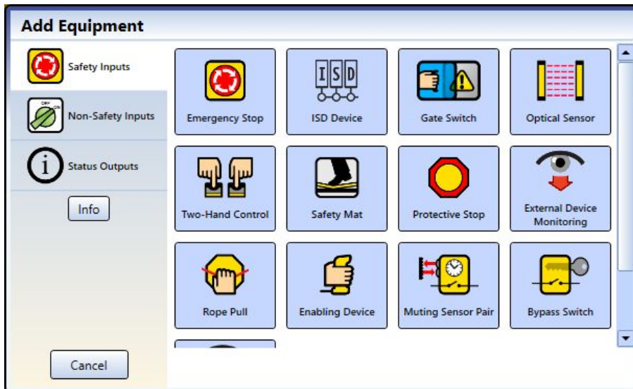
Figure 56. SC10-2: Adding inputs from Equipment View (physical status output can only be added from this view)
