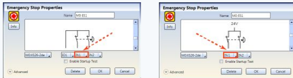
Figure 23. Manually Configured Circuits
