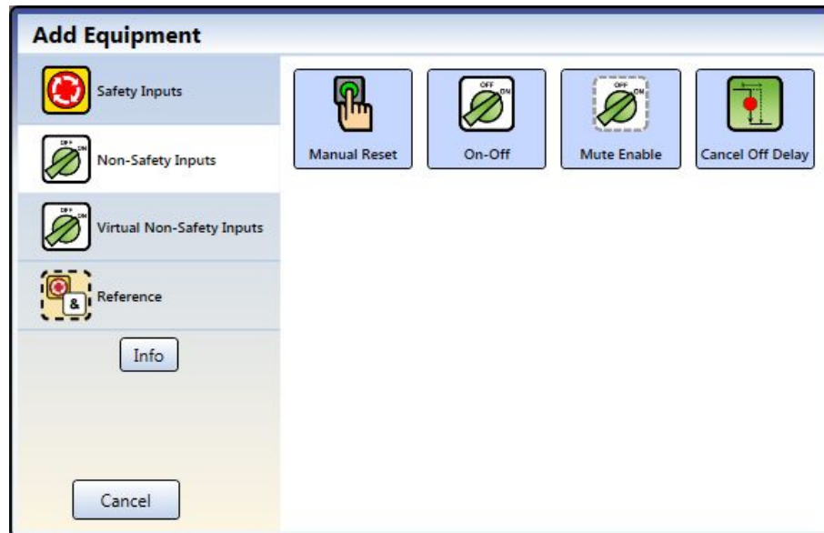
Figure 57. Non-Safety Inputs (Virtual Non-Safety Inputs available only from the Functional View Tab )
