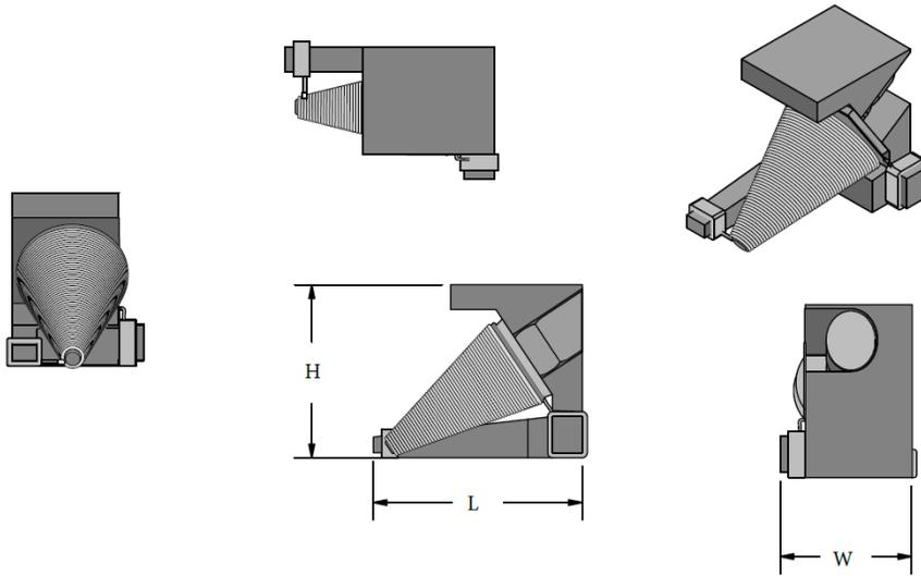
Note: Terminal is configured to facilitate attachment close to inductor tip.
