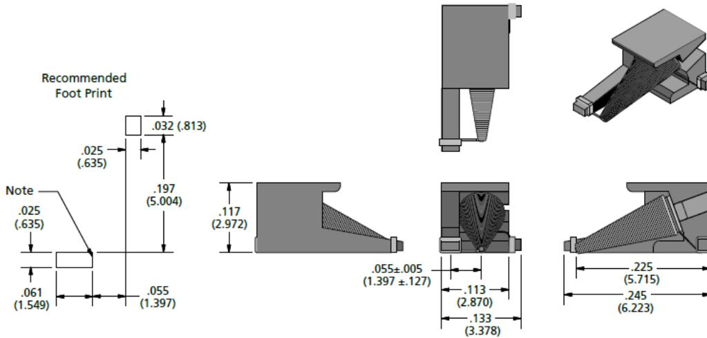
Note: Terminal is configured to facilitate attachment close to inductor tip.
