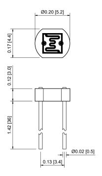
Note: Lead soldering temperature (1/16 inches away from body) 260°C for 3 sec.
