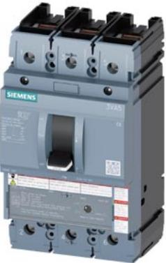
circuit breaker 3VA5 UL Frame 250 breaking capacity class C 100 kA @ 480 V 3-pole, line protection TM230, FTAM,  $I_n=110$  A overload protection  $I_r=110$  A permanently set short-circuit protection  $I_s=5\ldots 10 \times I_n$  UL 489 SB (naval), 50 degrees Celsius cable connection on two sides
