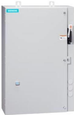
Non-reversing motor starter, Size 3, Three phase full voltage, Solid-state overload relay, OLR amp range 25-100A, 110V 50Hz / 120V 60Hz coil, Combination type, 100A fusible disconnect, 100A/250V fuse clip, Encl NEMA type 4X 304 S-Steel, Water/dust tight noncorrosive, Standard width enclosure
