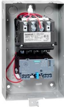
Non-reversing motor starter, Size 00, Three phase full voltage, Solid-state overload relay, OLR amp range 0.75-3.4A, Non-combination type, Enclosure type 1, Indoor general purpose use, Standard width enclosure
