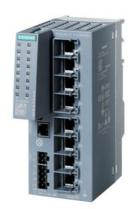
SCALANCE XC208G EEC manageable Layer 2 IE switch; IEC 62443-4-2 certified; 8x 10/100/1000 Mbit/s RJ45 ports; 1x console port; diagnostics LED; redundant power supply; with painted printed-circuit boards; NAMUR NE21-compliant; temperature range -40 °C to +70 °C; assembly: DIN rail/S7 mounting rail/wall; redundancy functions; Office features (RSTP, VLAN,...); PROFINET IO device; Ethernet/IP-compliant; C-plug slot;
