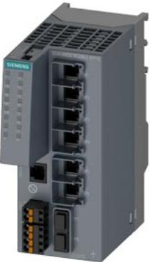
SCALANCE XC206-2SFP G (E/IP) manageable Layer 2 IE switch; IEC 62443-4-2 certified; 6x 10/100/1000 Mbps RJ45 ports; 2x 1000 Mbps SFP; 1x console port; diagnostics LED; redundant power supply; temperature range -40 °C to +70 °C; assembly: DIN rail/S7 mounting rail/wall; redundancy functions; office features (RSTP, VLAN,...); PROFINET IO device; Ethernet/IP-compliant; C-PLUG slot; default EtherNet/IP. IEEE 1588v2 PTP
