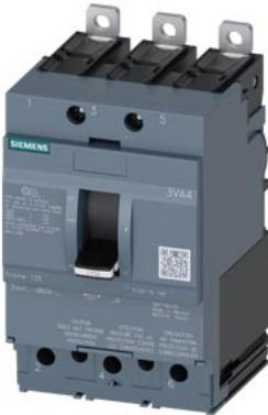
molded case switch 3VA4 UL frame 125 max. sh-circ breaking capacity 65kA @ 480 V 3-pole, line protection MCS110, In=100A without overload protection self-protection li=16 x In clamp connection
