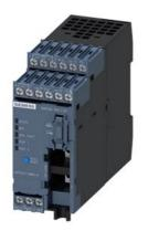
basic device SIMOCODE pro V EIP, EtherNet/IP, media redundancy, DLR (max. 20 participants) web server, transfer rate 100 Mbps, 2 x bus connection via RJ45, 4 l/3 O freely configurable, Us: 24 V DC, input for thermistor connection monostable relay outputs, expandable by expansion modules
