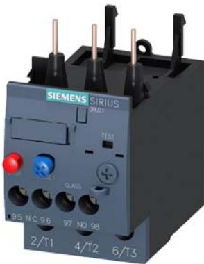
Overload relay 9.0...12.5 A Thermal For motor protection Size S0, Class 10
