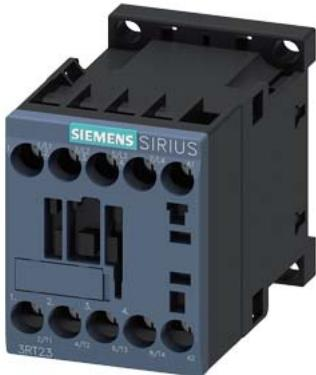
contactor AC-1, 18 A, 400 V / 40 °C, 4-pole, 220 V AC, 50 Hz / 240 V, 60 Hz, screw terminal, size: S00
