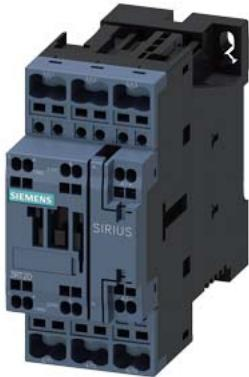
traction contactor, AC-3e/AC-3, 38 A, 18.5 kW / 400 V, 3-pole, 125 V DC, 0.7-1.25\* Uc, solid-state operating mechanism, with integrated varistor, auxiliary contacts: 1 NO + 1 NC, spring-loaded terminal, frame size: S0
