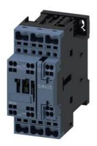
power contactor, AC-3e/AC-3, 32 A, 15 kW / 400 V, 3-pole, 220 V AC, 50 Hz / 240 V, 60 Hz, auxiliary contacts: 1 NO + 1 NC, spring-loaded terminal, size: S0
