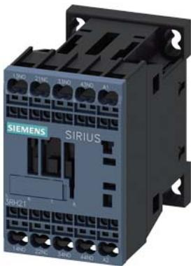
contactor relay, 3 NO + 1 NC, 110 V AC, 50/60 Hz, spring-loaded terminal, frame size S00
