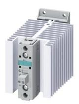
Solid-state contactor 1-phase 3RF2 AC 51 / 50 A / 40  $^{\circ}\text{C}$  48-600 V / 4-30 V DC screw terminal Blocking voltage 1200 V
