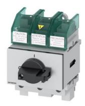
SENTRON 3LD5 switch disconnector UL, main switch, 3-pole, approved according to UL 489, UL 60947-4-1 and IEC 60947-3, UL: 60 A, SCCR 50 kA at 480 V AC, operational power @ 480 V AC 3-phase: 40 hp, IEC: 63 A, operational power at AC-23 A at 400 V: 30 kW, floor mounting with direct operating mechanism, black including terminal covers for the infeed side for the infeed side
