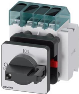
3LD3 switch disconnector, I<sub>u</sub> 63 A main switch 3-pole + N rated operational power at AC-23 A at 400 V 22.0 kW front plate mounting basic switch with center-hole mounting 22.5 mm knob-operated mechanism black 48x48 mm with auxiliary switches 1 NO + 1 NC
