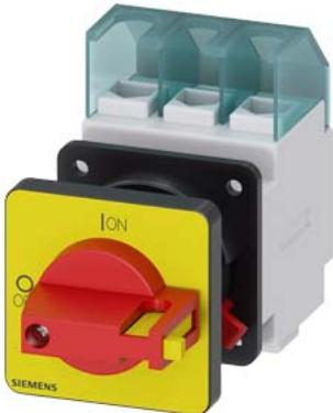
SENTRON, Switch disconnector 3LD, emergency switching-off switch, 3- pole, I<sub>u</sub>: 32 A, operating power / at AC-23 A 400 V: 11.5 kW, front-mounted, knob-operated mechanism, Red / yellow, central mounting 22.5 mm of the handle
