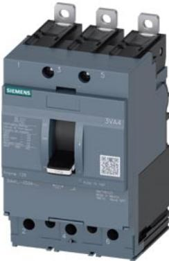
circuit breaker 3VA4 UL Frame 125 breaking capacity class M 35 kA @ 480 V 3-pole, line protection TM210, FTFM,  $I_n=15$  A overload protection  $I_r=15$  A permanently set short-circuit protection  $I_s=20 \times I_n$  UL 489 SB (naval), 50 °C, terminal connection
