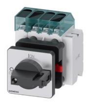
3LD3 switch disconnector, lu 32 A main switch 3-pole + N rated operational power for AC-23 A at 400 V 11.5 kW front plate mounting basic switch with center-hole mounting 22.5 mm knob-operated mechanism black 48x48 mm with auxiliary switches 1 NO + 1 NC
