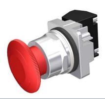
30mm Command/52, Chrome Finish Heavy Duty, Watertight/Oiltight Complete Metal Unit Twist-to-Release Operator Non-Illuminated Mushroom Head Cap Small 1.79" (45 mm) Plastic Cap, Red 2 Position Maintained, Twist-to-Release with 1 N.O. - 1 N.C. Heavy Duty Contacts, A600/P600 UL Listed, CSA Certified NEMA 1,3,3R,4,4X,12,13 & Automotive Standards
