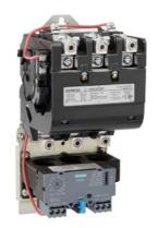
Non-reversing motor starter Size 3 Three phase full voltage Solid-state overload relay OLRelay amp range 25-100A 110VAC 50HZ / 120VAC 60HZ coil Combination type No enclosure
