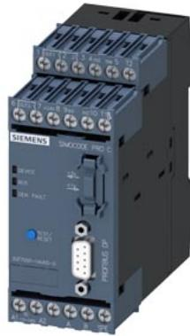
basic device SIMOCODE pro C, PROFIBUS DP interface 12 Mbps, RS-485, 4 I/O freely configurable, Us: 110...240 V AC/DC, input for thermistor connection monostable relay outputs
