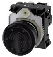
acoustic signal device, compact, 22 mm, round, plastic, black, continuous tone 4.5 kHz, IP69, sound pressure 75+/-10% dB/10 cm, with holder, operating voltage 24 V AC/DC. screw terminal
