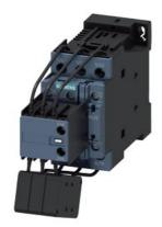
capacitor contactor, AC-6b 16.7 kVAr, / 400 V, 3-pole, 21-28 V AC/DC, 50/60 Hz, with integrated varistor, auxiliary contacts: 1 NO + 2 NC, screw terminal, size: S0
