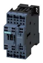
traction contactor, AC-3e/AC-3, 38 A, 18.5 kW / 400 V, 3-pole, 125 V DC, 0.7-1.25\* Uc, solid-state operating mechanism, with integrated varistor, auxiliary contacts: 1 NO + 1 NC, spring-loaded terminal, frame size: S0
