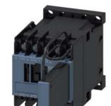
traction contactor, AC-3e/AC-3, 16 A, 7.5 kW / 400 V, 3-pole, 24 V DC, 0.7-1.25  $^{\star}$  Uc, with integrated suppressor diode, auxiliary contacts: 1 NC, ring cable lug connection, frame size: S00, with plugged on series resistor
