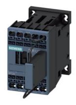
traction contactor, AC-3e/AC-3, 16 A, 7.5 kW / 400 V, 3-pole, 24 V DC, 0.7-1.25  $^{\star}$  Uc, with integrated suppressor diode, auxiliary contacts: 1 NC, spring-loaded terminal, frame size: S00, with plugged on series resistor
