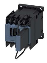
traction contactor, AC-3e/AC-3, 12 A, 5.5 kW / 400 V, 3-pole, 24 V DC, 0.7-1.25  $^{\star}$  Uc, with integrated suppressor diode, auxiliary contacts: 1 NC, ring cable lug connection, frame size: S00, with plugged on series resistor
