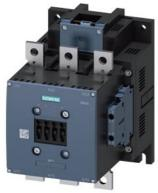
power contactor, AC-3e/AC-3 225 A, 110 kW / 400 V Uc: 24 V DC x (0.7-1.25) PLC input 24-110 V DC 3-pole, auxiliary contacts 2 NO + 2 NC drive: electronic main circuit: busbar control and auxiliary circuit: screw terminal extended rated condition railroad IEC 60077
