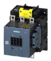
power contactor, AC-3e/AC-3 115 A, 55 kW / 400 V, AC (50-60 Hz) / DC Uc: 96-127 V x (0.8-1.1) F-PLC input 24 V DC 3-pole, auxiliary contacts 2 NO + 2 NC drive: electronic main circuit: busbar control and auxiliary circuit: screw terminal
