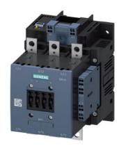
power contactor, AC-3e/AC-3 115 A, 55 kW / 400 V, Uc: 24 V DC x (0.7-1.25) PLC input 24-110 V DC 3-pole, auxiliary contacts 2 NO + 2 NC drive: electronic main circuit: busbar control and auxiliary circuit: spring-loaded terminal
