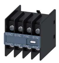
auxiliary switch, on the front, 1 NO + 3 NC, 53/54, 61/62, 71/72, 81/82, current path: 1 NO, 1 NC, 1 NC, 1 NC, ring cable lug connection, physically coded, only with contactor relays 3RH2140 and 3RH2441 combinable (according to EN 50011)
