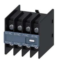
auxiliary switch, on the front, 4 NC, 51/52, 61/62, 71/72, 81/82, current path: 1 NC, 1 NC, 1 NC, 1 NC, ring cable lug connection, physically coded, only with contactor relays 3RH2140 and 3RH2440 combinable (according to EN 50011)
