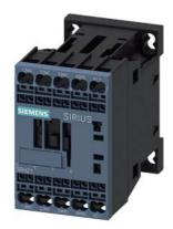
contactor relay, 3 NO + 1 NC, 24 V DC, with integrated diode, spring-loaded terminal, frame size S00,  $\,$
