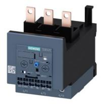
Overload relay 32...115 A Electronic For motor protection Size S3, Class 5E...30E Contactor mounting Main circuit: Screw Auxiliary circuit: Spring-type terminal Manual-Automatic-Reset
