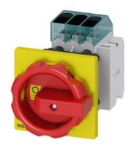
3LD3 switch disconnector, Iu 32 A main switch 3-pole rated operational power for AC-23 A at 400 V 11.5 kW front plate mounting basic switch with center-hole mounting 22.5 mm rotary operating mechanism red/yellow 66 x 66 mm with auxiliary switches 1 NO + 1 NC
