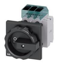
3LD3 switch disconnector, Iu 32 A main switch 3-pole rated operational power for AC-23 A at 400 V 11.5 kW front plate mounting basic switch with center-hole mounting 22.5 mm rotary operating mechanism black 66 x 66 mm with auxiliary switches 1 NO + 1 NC
