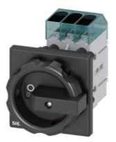
Load disconnector 3LD3, Iu 16 A Main switch 3-pole Rated operating capacity at AC-23 A at 400V 7.5kW Front plate mounting Basic switch with Central hole mounting 22.5mm Rotating drive black 66 x 66 mm
