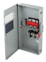
Siemens Low Voltage Circuit Protection Heavy Duty Safety Switch. 3-Pole 3-Fuse and solid neutral Fused in a type 3R enclosure (outdoor). Rated 240VAC (400A).
