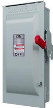
Siemens Low Voltage Circuit Protection Heavy Duty Safety Switch. 3-Pole 3-Fuse and solid neutral Fused in a type 3R enclosure (outdoor). Rated 240VAC (100A).
