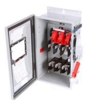
Siemens Low Voltage Circuit Protection Heavy Duty Safety Switch. 3-Pole 3-Wire Fused in a type 12 industrial enclosure. Rated 240VAC (100A). Special features: Crouse-Hinds interlocked receptacle.
