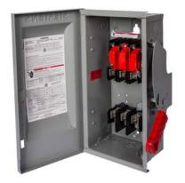
Siemens Low Voltage Circuit Protection Heavy Duty Safety Switch. 3-Pole 3-Fuse and solid neutral Fused in a type 3R enclosure (outdoor). Rated 240VAC (60A). Special features: factory installed ground bar.
