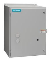
Mechanically held Lighting contactor Contactor amp rating 200Amp 0 NC / 3 NO poles 24VAC 60HZ coil Non-combination type Enclosure NEMA type 12 Dust/drip proof for indoors
