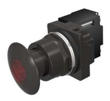
30mm BlackMax, Epoxy Coated Corrosion Resistant Complete Metal Unit Illuminated Push-Pull Operator Full Voltage, 120V AC/DC LED Lamp Mushroom Head Cap Small 1 3/4" (44.5 mm) Metal, Black with Red Lens 3 Position Momentary UL Listed, CSA Certified NEMA 1,3,3R,4,4X,12,13 & Automotive Standards
