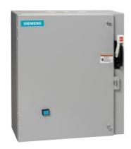
Non-reversing motor starter Size 2 1/2 Three phase full voltage Solid-state overload relay OLRelay amp range 25-100A 380-440/440-480V 50/60HZ coil Combination type 100A fusible disconnect 100A/250V fuse clip Enclosure NEMA type 1 Indoor general purpose use Standard width enclosure
