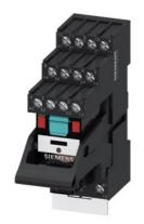
plug-in relay complete unit, 4 changeover contacts, 115 V AC, LED module red, base with logical isolation, screw terminal, 3.5 mm pinning
