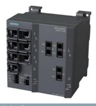
SCALANCE X307-3LD, managed plus IE switch, 3x 1000 Mbit/s SM SC 7x 10/100 Mbit/s RJ45 ports, LED diagnostics, error-signaling contact with Select/set pushbutton, PROFINET IO Device, network management, integrated redundancy manager, Office features (RSTP, VLAN, IGMP,...) C-plug in scope of delivery .
